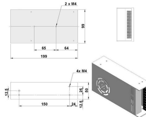
12VDC 25A: 199 (L) ×99 (W) ×50 (H) mm<sup>3</sup>, 0.9 kg
