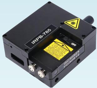
Changchun New Industries (CNI) imaging Raman probe integrates a standard Raman probe with an imaging optical path into a visual Raman probe. The imaging function displays the laser excitation spot, facilitating alignment of the sampling position. The camera can be connected to a computer via a USB interface.
