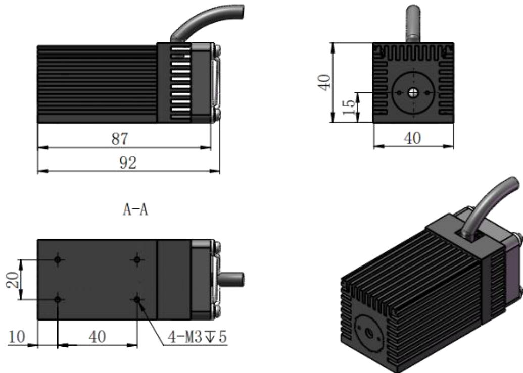
Dimensions of PSU-V-OEM power supply
