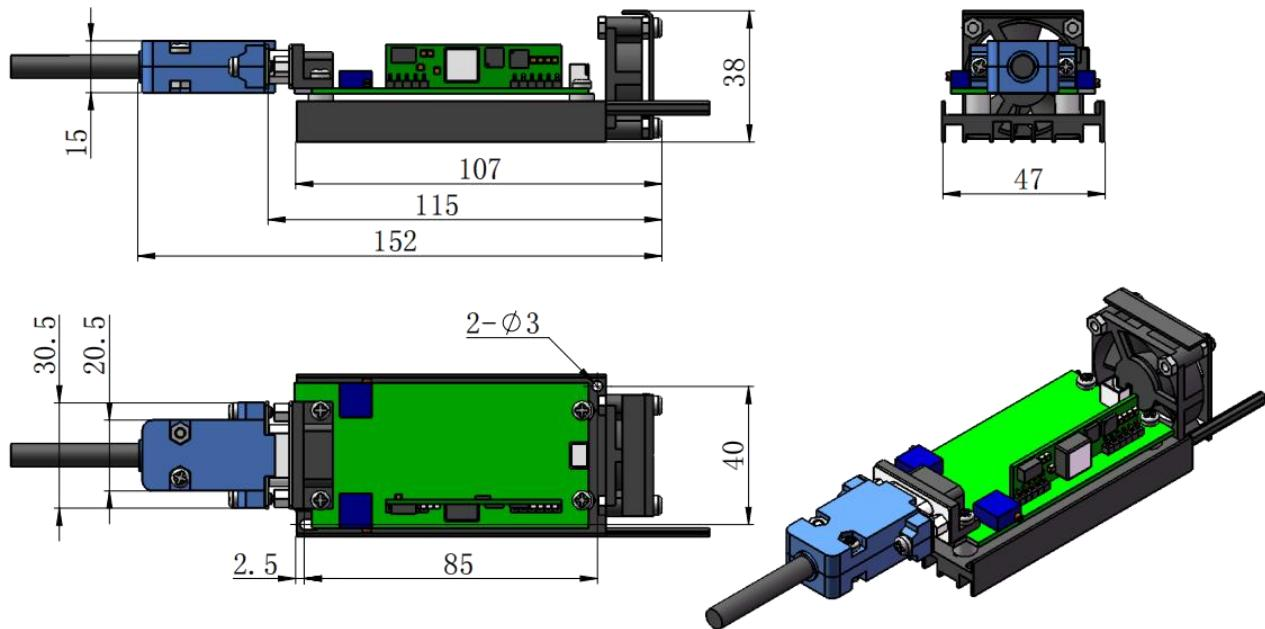
Dimensions of PSU-V-OEM and PSU-I-OEM power supply with dust cover( $110 \times 70 \times 47\text{mm}^3$ )
