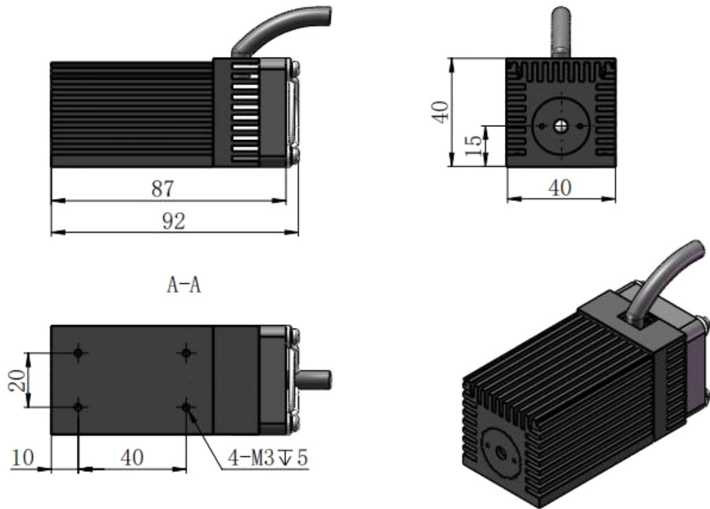
Dimensions of PSU-V-OEM power supply
