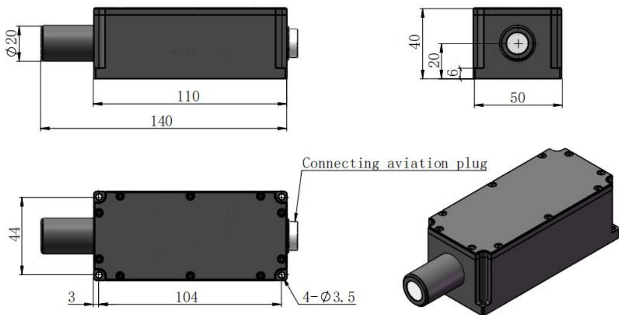
Dimensions of laser (PCB integrated & adjustable focusing distance) (mm):
